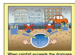
When rainfall exceeds the drainage capacity of sewers, water overflows from sewers or the water which cannot enter sewers remains on the ground.
